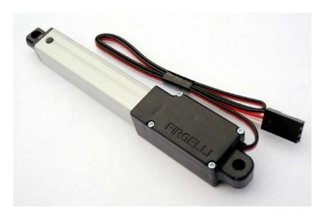
The L12-R servo is designed to work with all common RC Transmitter and Receiver Pairs. The most important thing to check is that the power supplied to the actuator is between 5VDC and 7VDC. The red wire is 6v power, black is ground and white is the PWM RC signal wire. The L12-R accepts pulse widths signals from 1-2ms.
